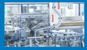
Feeding unit for bottles so that they can be serialized on the BEC 200's cartoner and packed in folding boxes
