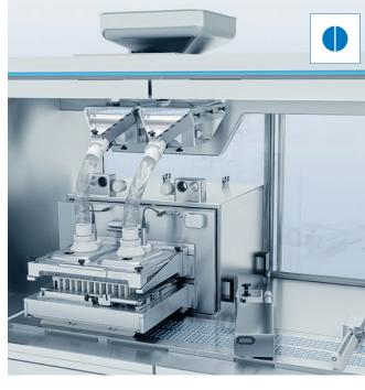
The **SimTap 4 feeder** feeds a wide variety of solid product shapes into the film pockets reliably, gently and precisely. A brush-in box can be attached to the basic module of the SimTap 4 in just a few steps. This means that two feeding principles can be implemented with one basic module – for particularly economical and efficient packaging.
