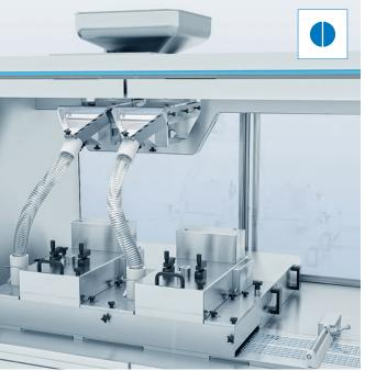
The **brush-in feeder** is suitable for thermoforming foils and can be used on both continuous and intermittent blister machines.
