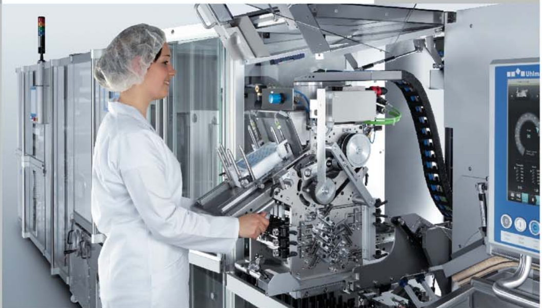
Right: The leaflet folder, which can be pulled forward and turned.
